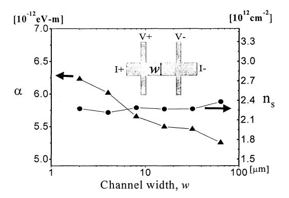
Fig. 1 Channel width dependence of spin-orbit interaction parameter and carrier concentration
