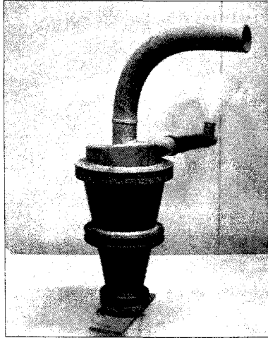
Fig. 2 The tribo-charger of cyclone type used this study.
