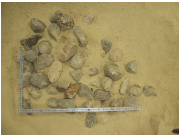
Fig. 5. CASE 1. The mean dimension of rocks is 8cm
