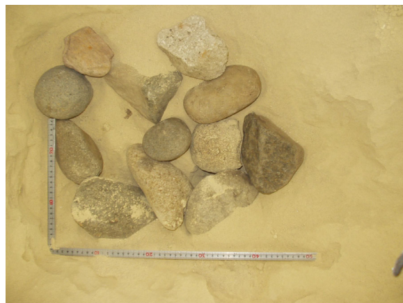
Fig. 6. CASE 21. The mean dimension of rocks is 15cm
