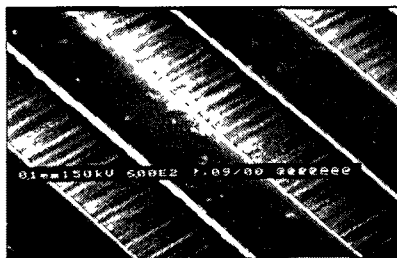
Figure 4 A SEM photo of test pattern on copper plate. The DFR is 405 nm sensitive.
