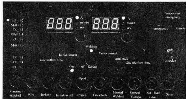
Fig. 1 Main operating panel
