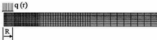
Fig. 1 Mesh design and loading condition for laser efficiency
