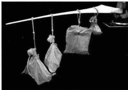
Fig. 9 Static test of the prototype blade
