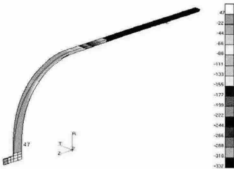
Fig. 5 Minimum principal stress distribution at 0 pressure after autofretage.
