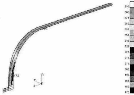
Fig. 4 Von-Mises stress distribution at autofretage pressure (35.7MPa).
