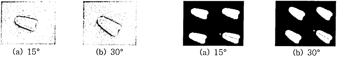
Fig. 4 Input image from CCD camera and results of image processing according to gradient of chambak
