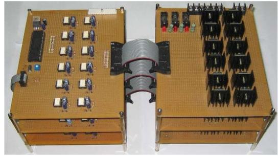
Fig. 4 Three phase multi-level inverter
