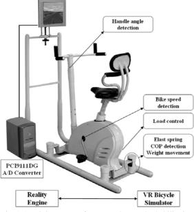
Fig. 1 A training system for postural control rehabilitation
