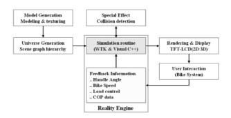
Fig. 4 Block diagram of the virtual bicycle simulator software
