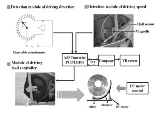
Fig. 3 The major mechanical parts of the virtual bicycle system
