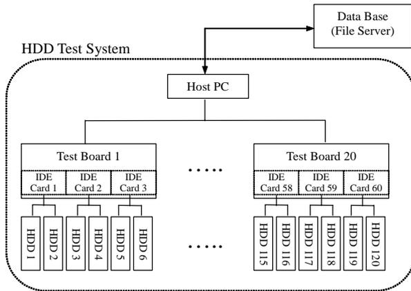
Fig. 2. Architecture of a HDD Test System
