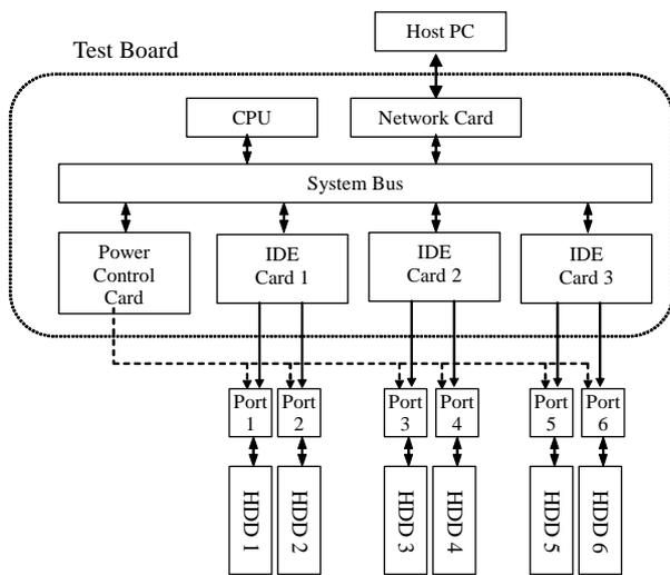
Fig. 3. Architecture of a Test Board
