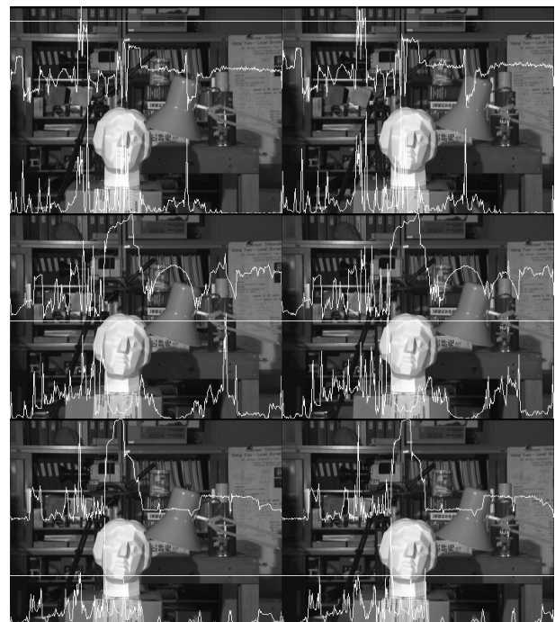
Fig. 4 Edge projection and brightness distribution along row. White line shows corresponding row in the image, and upper profile is the brightness and lower profile is edge projection (From left to right: left image and right image).
