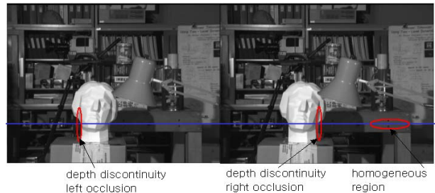
Fig. 1 Difficulty in stereo matching: depth discontinuity, occlusion and homogeneous region.
