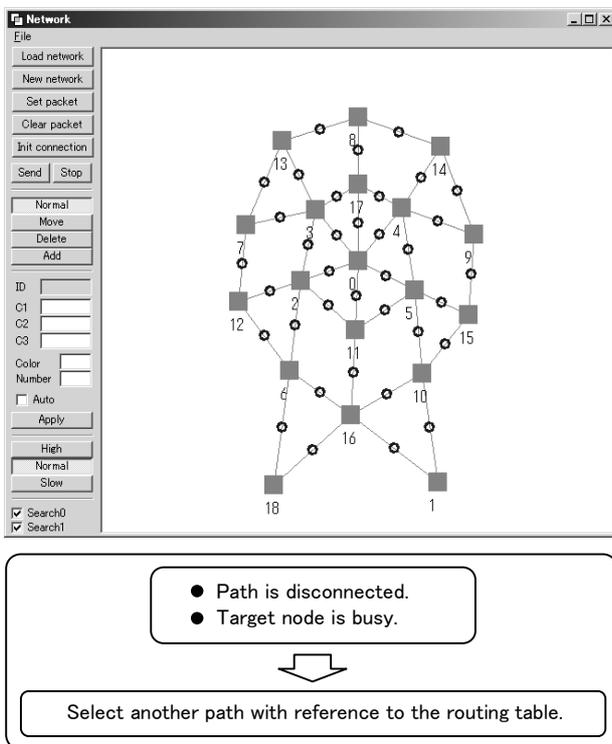
Figure 13. Computer simulation of the decentralized network connection
