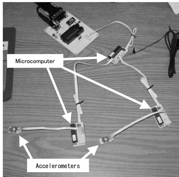
Figure 11. Prototyped network of acceleration sensor
