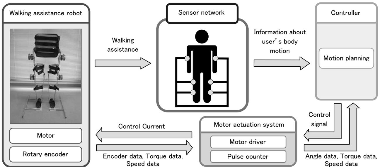
Figure 2. Control system of the walking assistance robot
