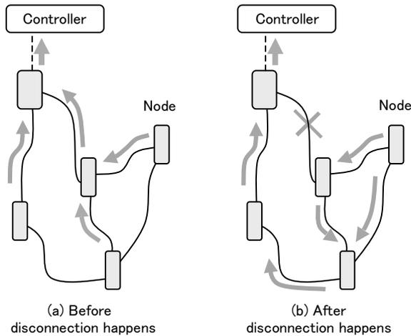
Figure 12. A sketch of the decentralized network connection
