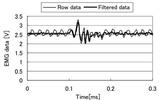
Figure 10. Experimental result of the adaptive self-tuning filter
