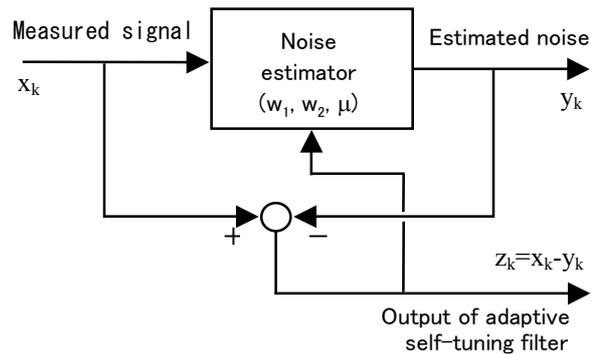
Figure 9. Block diagram of the adaptive self-tuning filter
