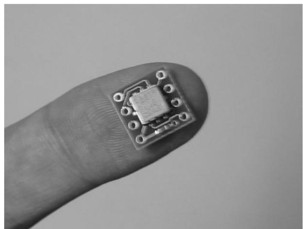
Figure 7. Accelerometer (ADXL202, Analog Devices, Inc)
