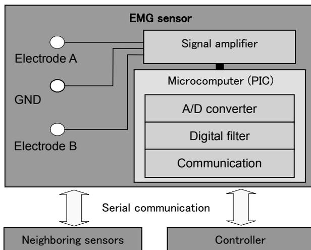
Figure 6. Configuration of the EMG sensor
