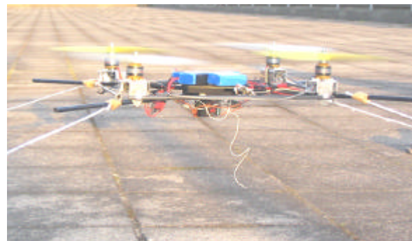
Fig.9 Motor test of four-rotor platform
