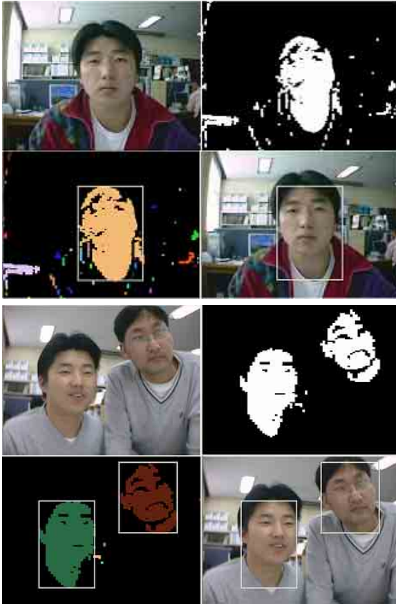
Fig. 7 Face candidate detection. Input image, skin color segmented and opening image, labeling image and face candidate images
