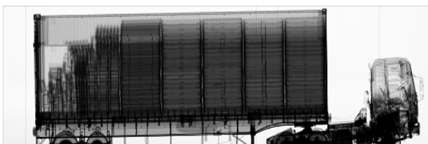
Fig. 4 X-ray inspection image of container truck (BMP format, 5169 \times 1262 size, 19,574,784 Bytes)
