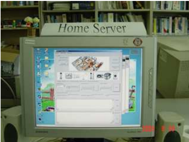
Fig. 3. HNCP home server implemented on a PC
