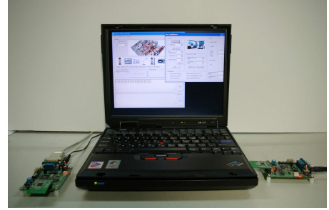
Fig. 10. Demonstration of wireless HNCP home network system based on the IEEE 802.15.4
