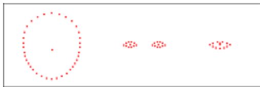
(a) Face (b) Eyes (c) Lips Fig. 3 Control points of the deformable template
