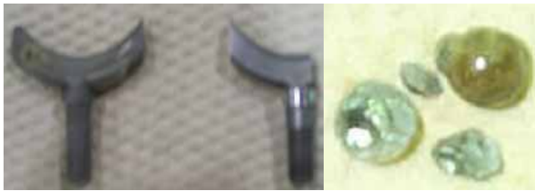
Fig. 2 Damaged deflector rods and balls
