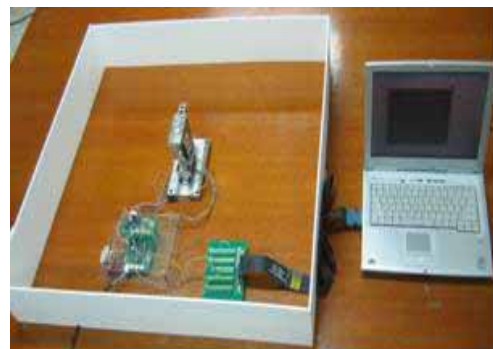
Fig. 5 Developed range finder system.
