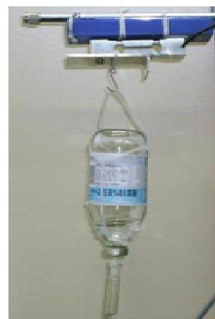
Fig. 5 Installation of the bottle of ringer s solution on loadcell
