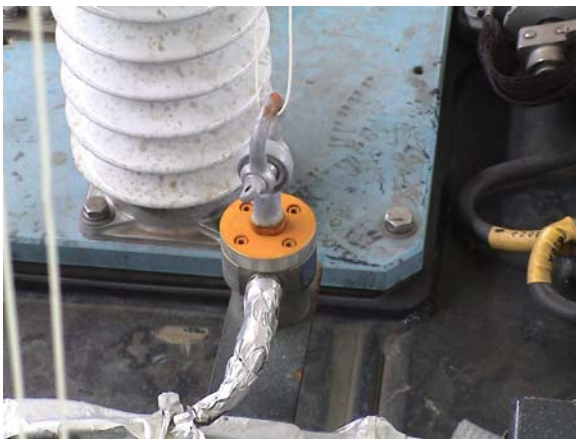
Figure 5 Load cell to measure lifting force
