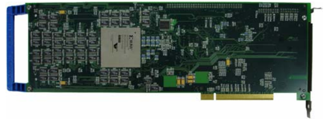
Fig. 5 The RC1000 board with a Virtex 2000E FPGA chip
