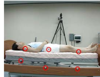
Fig. 7 Attached reflective markers on body and bed for measuring body posture.
