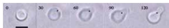
Fig. 4 Phase-contrast micrographs of the liposomes containing actin observed after the electroporation. Transformed liposomes obtained by the polymerization of encapsulated G-actin into F-actin. Number in each frame represents the time in sec elapsed after the pulse application. The symbol * indicates the reference point used to determine the rate of protrusive formation. The scale bars represent 10 \mu\text{m} .
