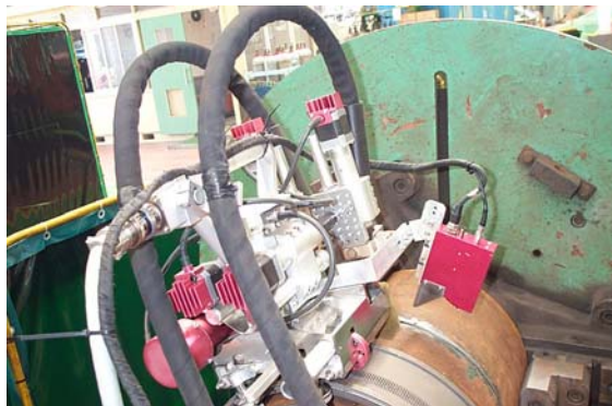
Fig. 11 Laser vision sensor developed
