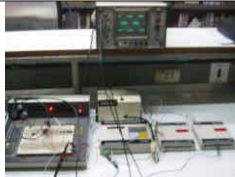
Fig.8 scan time measuring by oscilloscope
