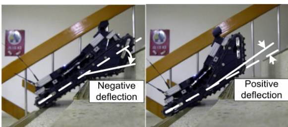
Fig. 4 Landform adaptability of passive mechanism
