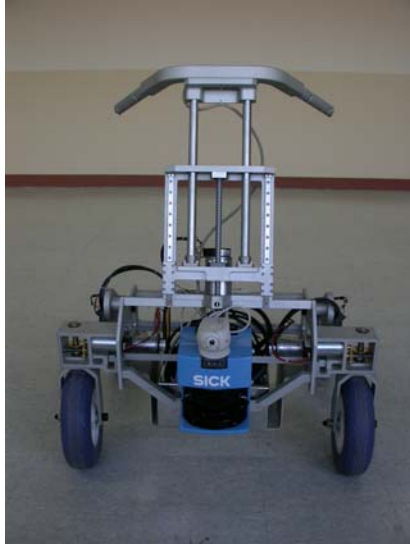
Fig. 1 The elderly assistance mobile robot with a haptic device and Touch Screen
