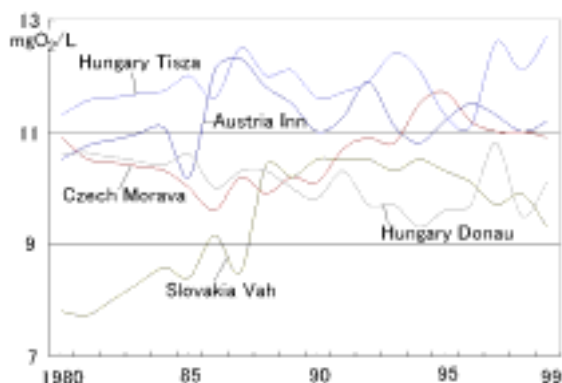
Fig.2 DO changes of Donau branches (the Inn, the Morava, the Vah, the Tisza) before BudaPest.
