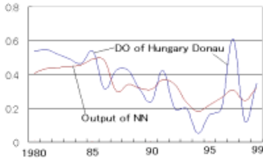
Fig. 5 DO of the Hungary Donau and output DO of a neural network in CQSAR. Both DOs are dimension-less. They are scaled in [0.05, 0.95], because of speed-up learning.
