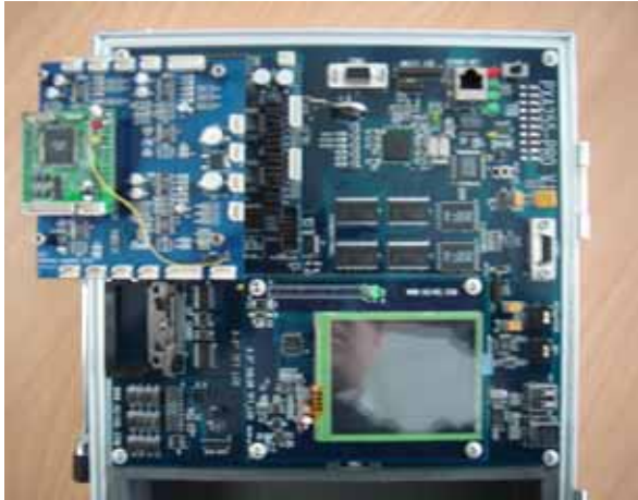
Fig.3 Programmable nonlinear amplification board on embedded system
