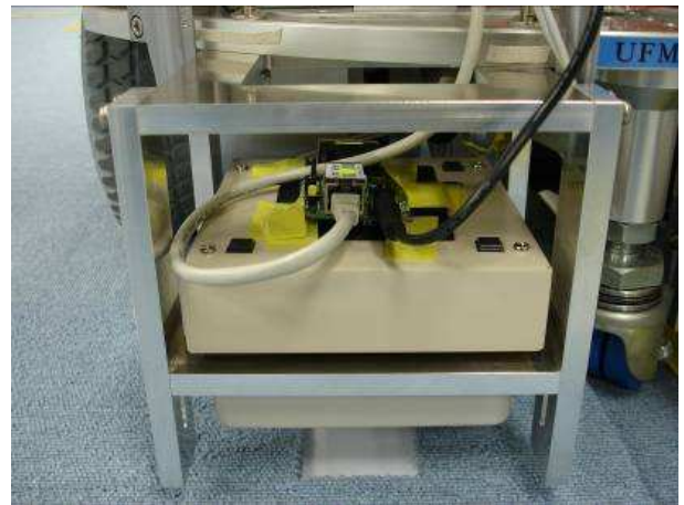
(b) RFID tag and reader (passive).
