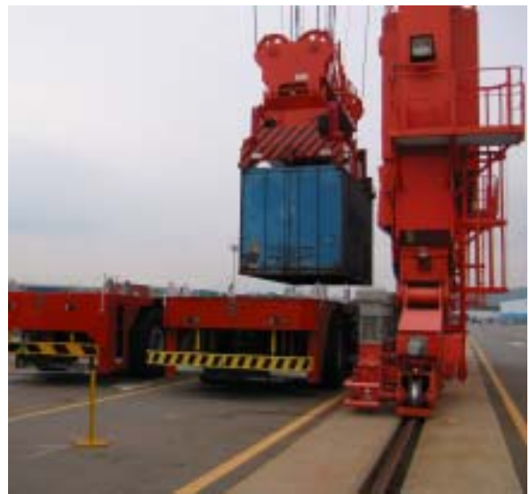
Fig. 8 AGV in automated container terminal
