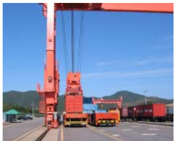
Fig. 9 AGV in automated container terminal
