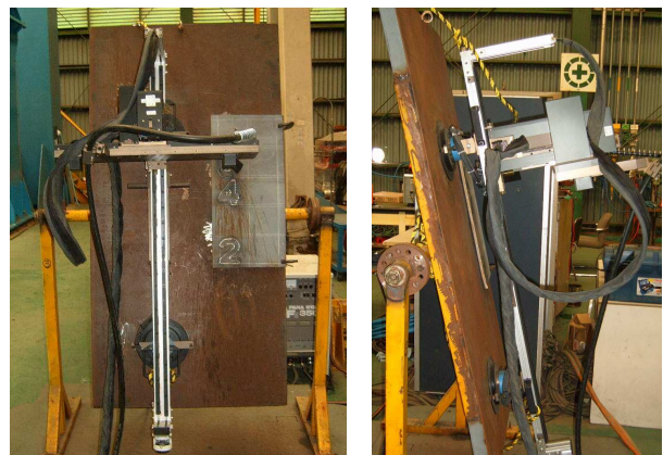
Fig. 10. Test bed for welding condition by angles
