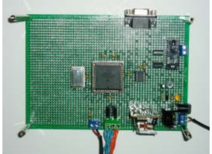
Fig. 9 Implemented control system board ( PIC18F6680).
