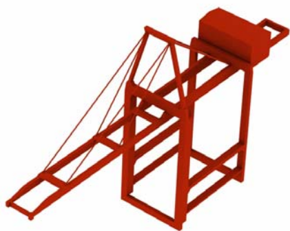
Fig. 1 3D configuration model of TTEC crane system.
