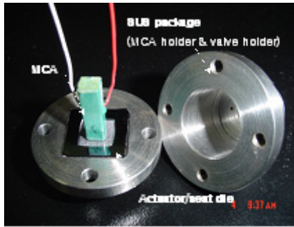
Fig. 4. Photograph of the fabricated MCA valve.
