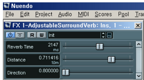
Fig. 4. Implemented software to adopt proposed reverberation algorithm
