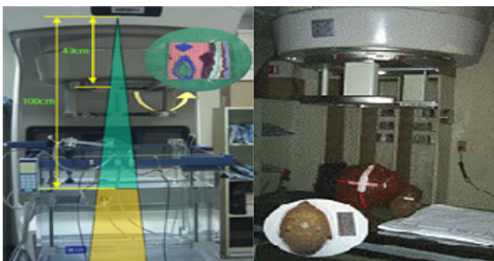
Fig. 7.(a) Water phantom setup (b) TLD setup
