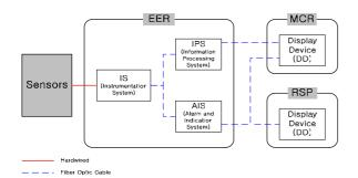
Figure 2. Monitoring interface between MCR and RSP
