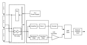
Fig 3. The simplified signal processing block diagram of Integral Reactor
