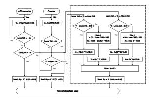
Fig 1. The signal flow
