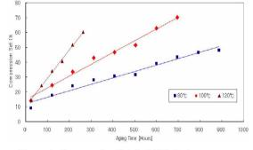
Figure 1. Compression Set for NBR O-ring
