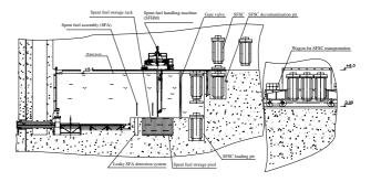
Figure 1. Spent fuel storage and handling scheme
