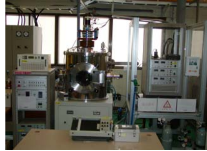
Figure 1. Ion beam sputtering system for making an experiment on improving the surface roughness of mold & die BLU(STAVAX).
