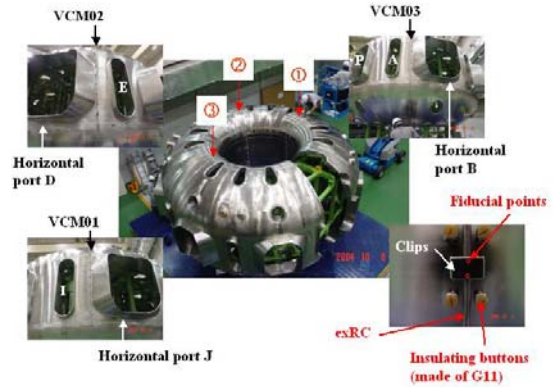
Figure 5. Three VCMs mounted on the external wall of the KSTAR machine.
