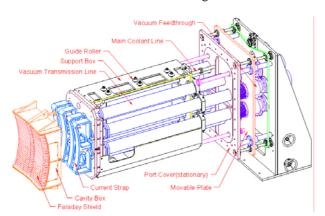
Figure 1. Detail 3-D drawing of the ICRF antenna.
