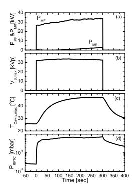
Figure 5. Time evolutions of the RF powers (a), line voltage (b), temperatures of the antenna cavity (c), and vacuum pressure of the RFTC (d) measured in long-pulse tests.
