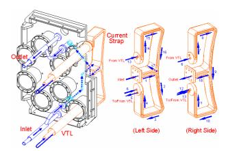
Figure 2. Cooling channels inside the current strap and the vacuum transmission lines.
