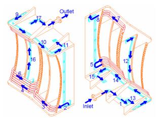
Figure 3. Cooling path diagram for the Faraday shield and the cavity walls.
