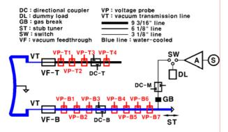
Figure 4. Schematic of the RF test circuit.
