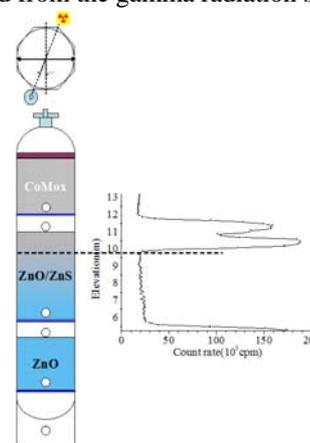
Fig.1 Vertical density profile of desulfurizing vessel by gross-counting method
