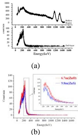
Fig. 2 (a) Comparison of scattered gamma spectra at empty and ZnO packed region, (b) Comparison of scattered gamma spectra at 9.8m (ZnS) and 6.7m (ZnO) in the reactor
