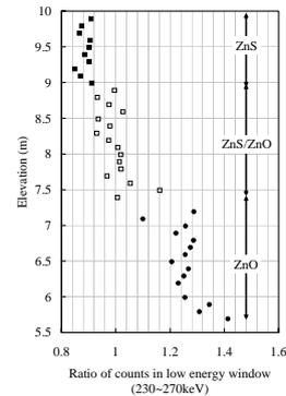
Fig. 3 Variation of relative count ratio in low energy window at various elevations
