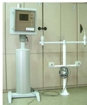
Figure4. Developed Environmental Radiation Monitoring System
